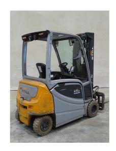
**Capacity:** 2000 kg YOM: 2018 **Running hours:** 6524 h **Engine type:** Electric Mast type: Triplex Closed height: 2160 mm Lift height: 4780 mm Fork length: 1000 mm Tyres: Super Elastic 2018 48V 625Ah **Battery:** Weight without battery: 2754 kg Storage BlackForxx Bremen
